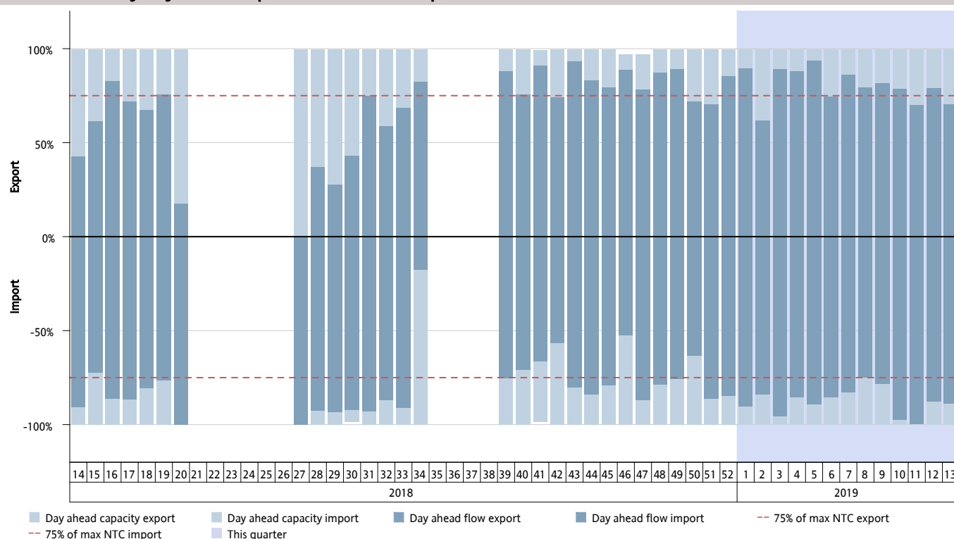
Figure 20: Shows cross-zonal day-ahead capacity result for the HVDC corridor DK2-DE, showing average weekly capacity given and flow as a percentage of max NTC. Available capacity is given for all hours, but the average flow is only given for hours with flow in that direction. Export indicates flow from DK2 to DE, while import indicates flow from DE to DK2.
