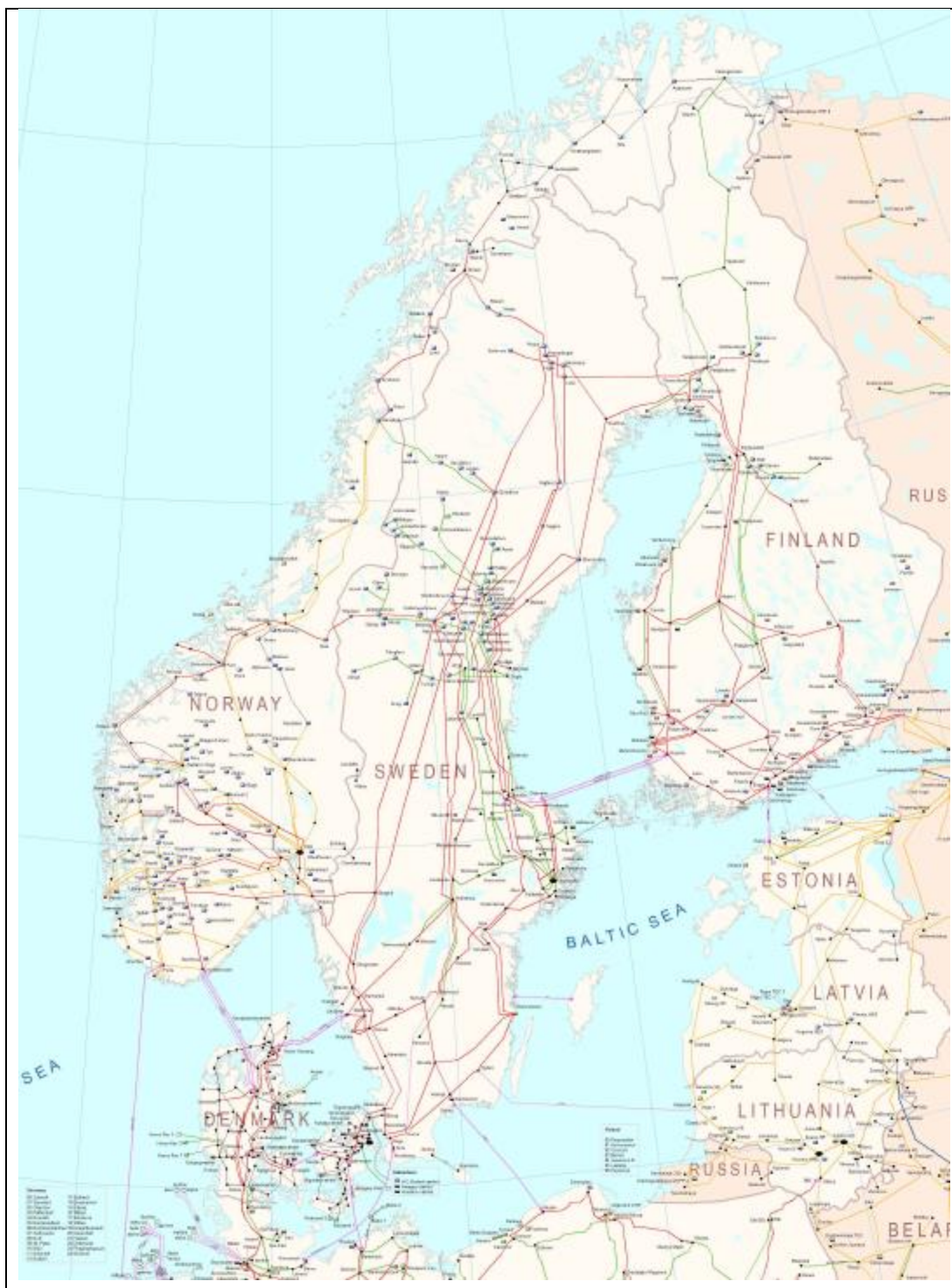
Figure 1 Map showing the Nordic power system (ENTSO-E, 2016). The transmission grid is needed to transport electric power from sites of generation to sites of consumption, but this grid has a limited capacity to transmit electric power.
